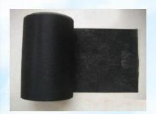
(Tested filter media with 4mm in thickness)
